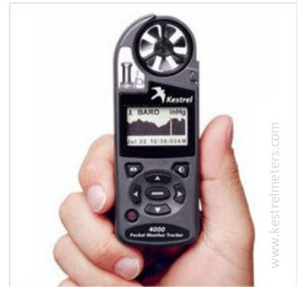
Handheld Kestrel sensor to measure thermal comfort
